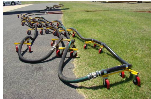
3 X 25 metre loading hoses and ramp skates.
